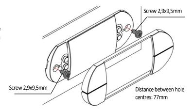
**Fig.3: NANO CHILL** console perforation template.
