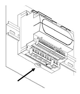
**Fig.2:** Fix the **NANO CHILL** console using the two screws to be inserted in the slots underneath the keys frame.
