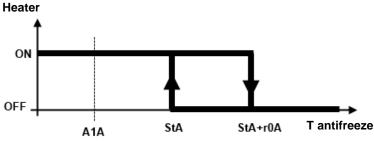
In this case the compressors are switched off to stop the refrigeration process, while the evaporator water pump remains active to avoid risks of freezing of the water inside the circuit. The antifreeze regulation is always active when the thermoregulation is active (if the probe is present and the resistors are present). If the chiller is in stand-by, it is possible to control the water in the circuit through the **PES** and **EPd** parameters.
