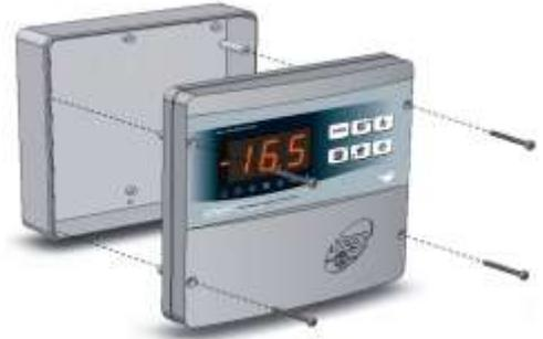
**Fig. 2:** Use the three existing holes to fix the box back panel to the wall: use three screws of a length suitable for the thickness of the wall to which the panel will be attached. Fit a rubber washer (supplied) between each screw and the box backing.
