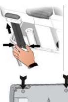
Fig. 6: Use the three existing holes to fix the box back panel to the wall: use three screws of a length suitable for the thickness of the wall to which the panel will be attached. Fit a rubber washer (supplied) between each screw and the box backing.
