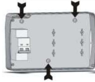
**Fig. 7:** Hook the frontal panel back up to the lower part of the box by inserting the two hinges in their seats and, bending them, rotate downwards 180° to gain access to the electronic board.
