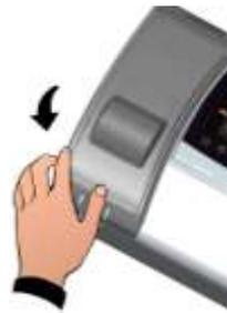
**Fig. 4:** Open the front of the box, lift it and slide the two hinges out as far as they will go.
