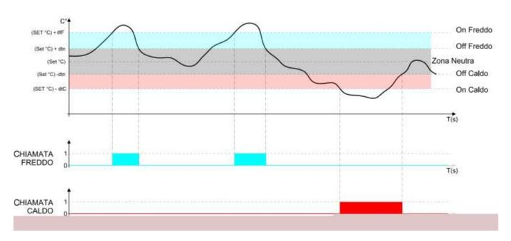
Parameter C1 introduces a delay between a switch-off and the subsequent re-activation of the cold. Hot can be deactivated with parameter EnH (EnH=0 disables the hot relay in all conditions).
