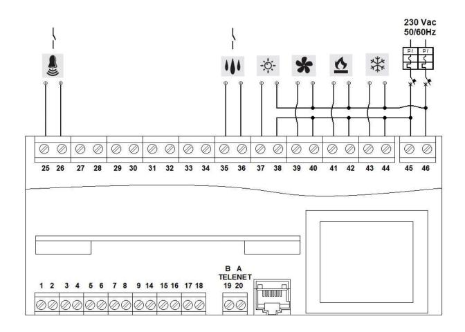
Example of electrical connection to the PLUS200 EXPERT THR with voltage contacts (230VAC) for compressor, heat, fans, light and contacts left without voltage for humidification and alarm.
