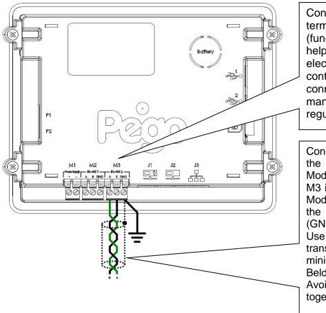
Connect the earth to the GND terminal of M3 in the console (functional earth). This connection helps to limit the effects of the electromagnetic noise on the control system. The ground connection must be made in a manner consistent with applicable regulations.
