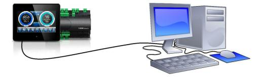
The network card of the computer must be configured to have the assignment of the DHCP address activated. In this case, the Vision Touch PAN and the computer, finding no DHCP server, will take the default IP addresses previewed for the class of addressing **169.254.xxx.xxx**. To connect to the device, it will be necessary to open a browser page and digit in the address bar the following order:
