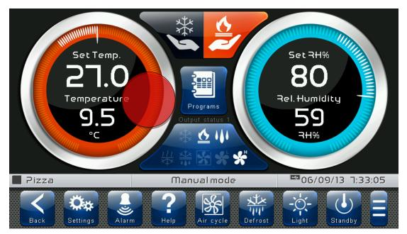
Once in modification mode, it is possible to change the humidity and temperature Set Points currently in use by turning the Wheel clockwise to increase or counterclockwise to decrease the value of the Set Point to be modified. Alternatively, you can use the plus and minus buttons. Furthermore, the speed of the fans can be changed using the buttons located in the center of the screen. Then confirm the new values with the green "Confirm" button or press "Cancel" to return to the display screen.
