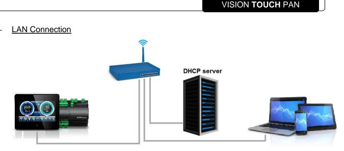
If connected to a LAN where a DHCP server is present (and the DHCP solicitude is enabled on the Vision Touch, look at chap. 8.3.9), the Vision Touch will acquire a free IP address. In this case it is possible to consult the IP address acquired through the "Info Page" that you find in the "Web server" menu of the Vision Touch.
