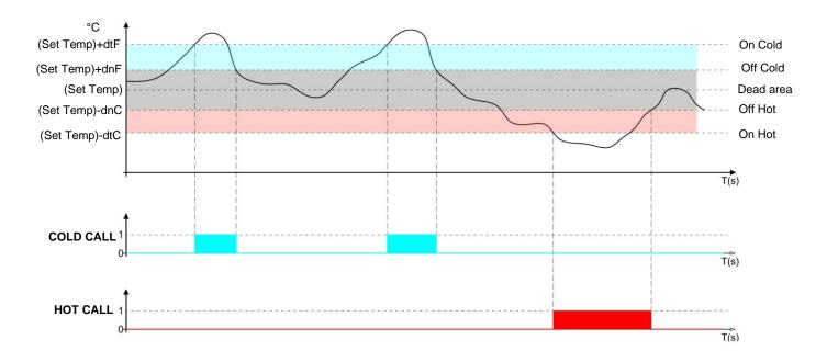
Parameter C1 (in "Parameters > Machine protection introduces a delay between a switchoff and the subsequent re-activation of the cold. Hot can be deactivated with parameter EnH in "Parameters > Configure PAN" (EnH=0 disables the hot relay in all conditions). Cold can be deactivated with parameter EnC in "Parameters > Configure PAN" (EnC=0 disables the cold relay in all conditions).
