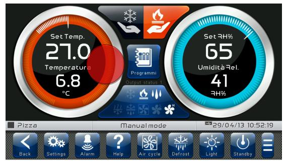
Edit Home 1 Page, Change Set Point with Wheel: Once you have entered edit mode on Home 1, it is possible to change the humidity and temperature Set Points currently in use. The variations are temporary and do not alter the preset program. Turn clockwise to increase or anti-clockwise to decrease the value of the Wheel of the Set Point to be modified or else act on the plus or minus buttons. Then confirm the new values by pressing the green confirmation button.
