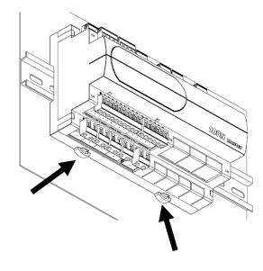
**Fig. 2:** Fix the **VISION 2PLT** console using the two screws to be inserted in the slots underneath the keys frame.
