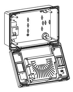
Fig. 4: Using the three pre-existing holes fix the bottom of the box with three screws of adequate length in relation to the thickness of the wall on which to fix the frame. Place a rubber washer (supplied) between each fixing screw and the bottom of the case. Then reassemble the battery (if present).
