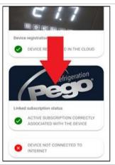
14) Touch the last link at the bottom "DEVICE NOT CONNECTED TO THE INTERNET" to configure the connection.
