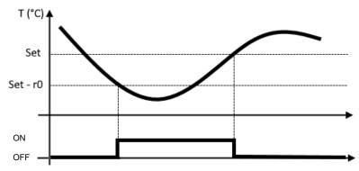
Compressor output or aux output configured as hot call (parameters AU1 / AU2)
