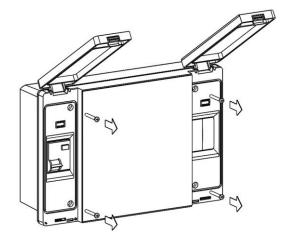
**Fig. 3:** Open the front of the box by lifting it and sliding the two hinges to the end of the stroke. Bend the hinges and rotate the front 180° downwards to access the inside of the panel.
